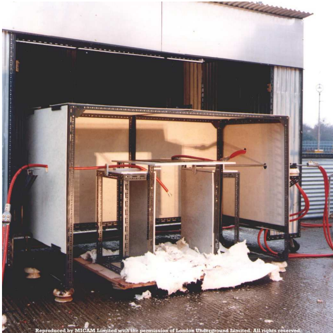
DC Arc Rig Prior To Test - View From The Front
